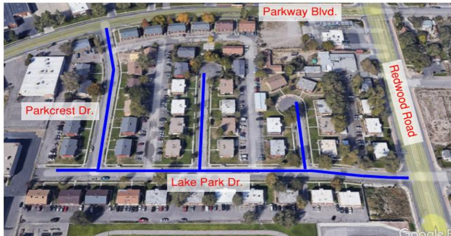
Replacement of 2,115 feet of 6" cast iron pipe from 1971 and 1977.
