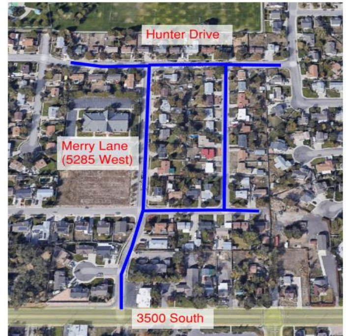
Replacement of 3,085 feet of 6" cast iron pipe from 1959 and 1970.
