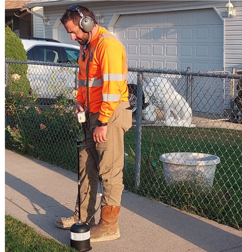
Figure 1: Kasey Newbold using the District's leak detection equipment to identify the location of a leak.
