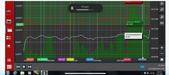
Temperature monitoring during curing of liner.
